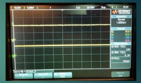
5V 4A Buck converter output (Odroid) Unloaded: 6.3V RMS .6 Vpp Loaded: 5V RMS .1 Vpp
